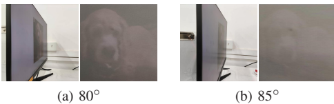
Fig. A4. The phenomenon of contrast drop at large angles. (a) and (b) are the shot images at 80° and 85° respectively.
