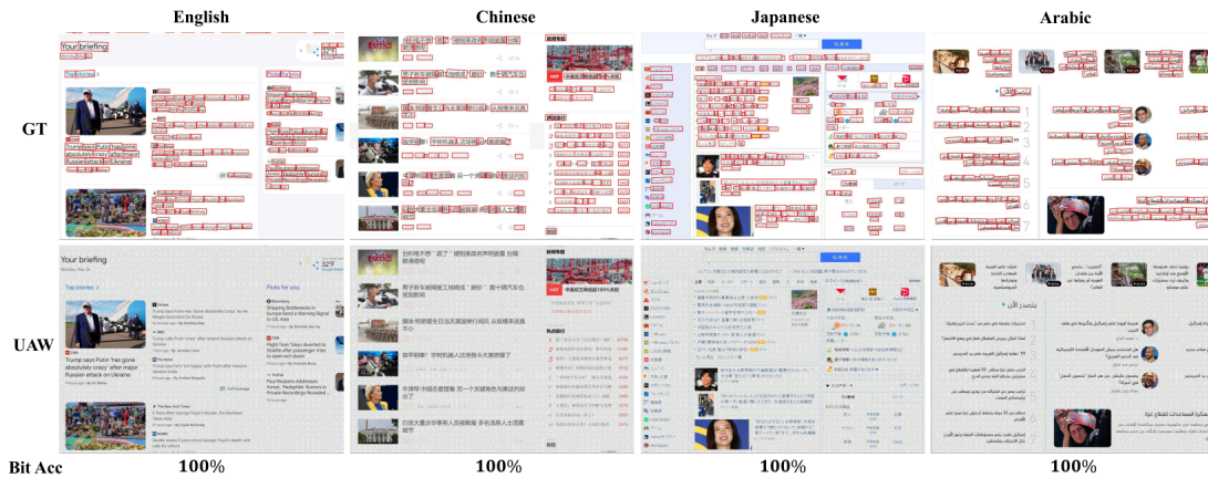
Fig. 13. UAW applied to web pages in different languages. Despite being trained only on English, UAW remains effective on Chinese, Japanese and Arabic. Watermark bit accuracy remains at 100% across all languages.
